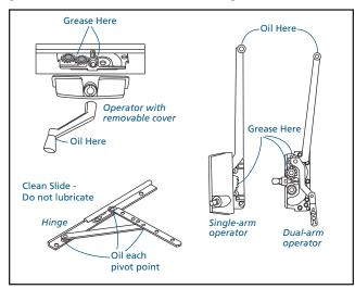
There are two types of operators with gear mechanisms:
